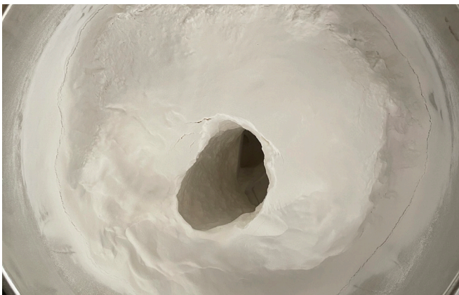
Benecel™ CR HPMC shows erratic flow and forms a rathole quite soon.
